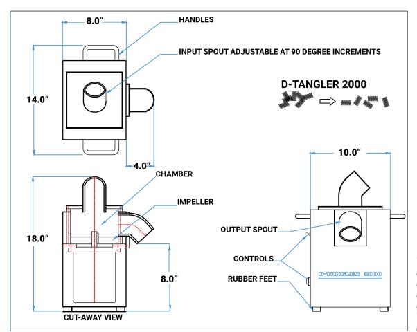
Weight: 45 lbs Power: 115VAC Hertz: 60 Phase: single Height: 18 inches Width: 12 inches No Pneumatics Required
